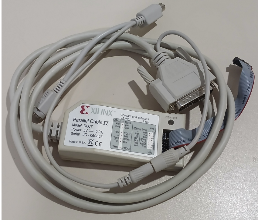
Figure 4.3: Power and data cables used in a Xilinx Spartan-3 development setup
