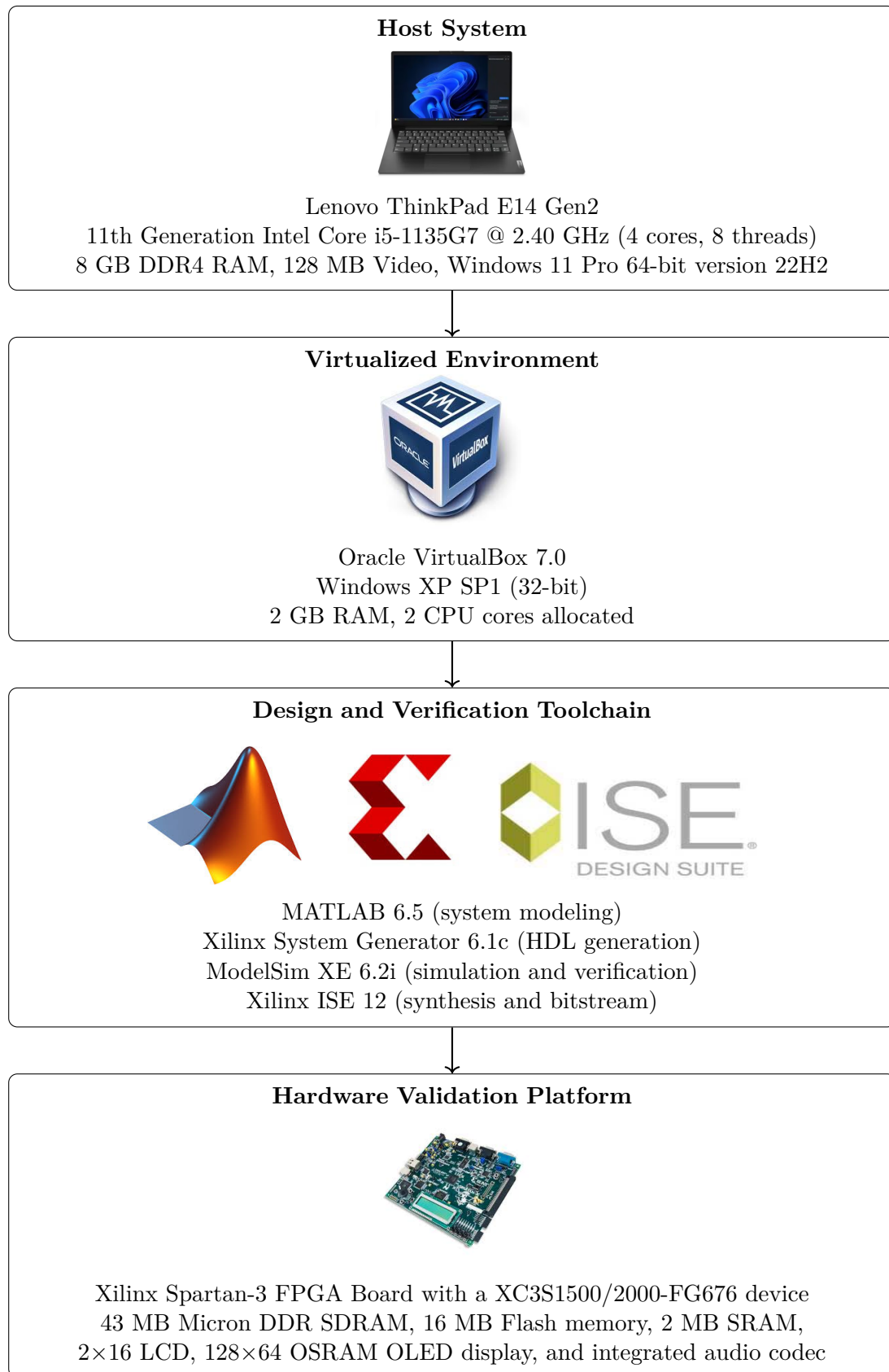
Figure 4.4: Experimental setup used for the design, simulation, and validation of the proposed solution.
