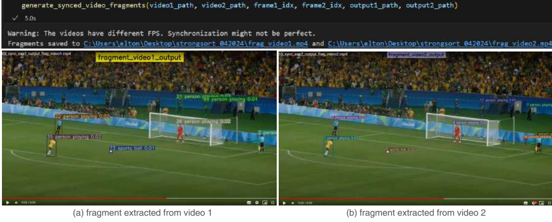
Figure 6.20: Synchronized video fragments generated automatically based on the visual features extracted by the MOT-UGV.
