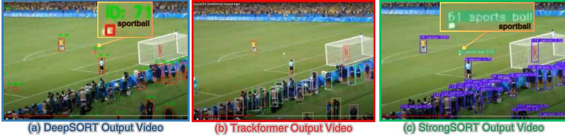
Figure 6.7: MOT Implemented - Output Videos: (a) DeepSORT (YOLO-v5), “sports ball” class detected; (b) TrackFormer result, no ball detected; (c) StrongSORT result, detected the “sports ball” class and improved tracking of multiple objects, including a person positioned near the goal area.
