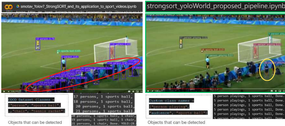
Figure 6.10: StrongSORT results: on the left YOLOv7 detected an average of 20 objects per frame. On the right, YOLO-World detected about 5 objects per frame, focusing mainly on those in the field.
