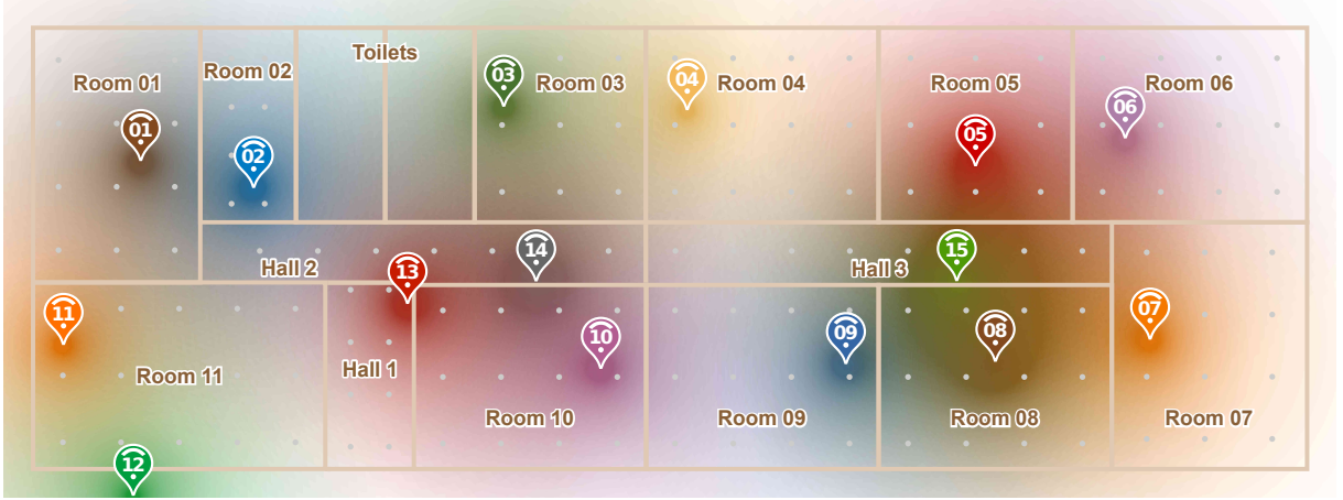
Figure 4 – Signal characterization of the environment using the signal propagation model as executed by the RSSI simulator.
