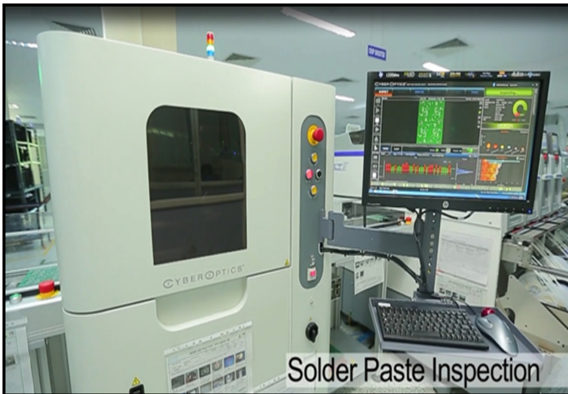
Figura 26 - SPI (Solder Paste Inspection)
